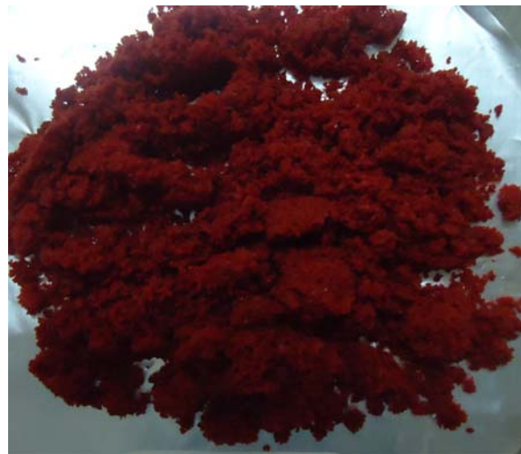
Fig 10: Gac powder with carrier: Gac seed membrane (1:1), maltodextrin: gelatin (0.5: 0.5), 2000ppm vitamin C
