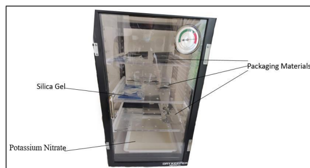
Fig 3: Accelerated Shelf-Life Testing (ASLT) Set-up
