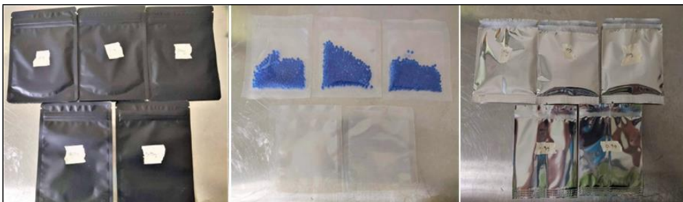
Fig 2: Different Packaging Materials used, a) MOPP/PET/AL/PE; b) NYLON/PE; and c) VMPET/PE
