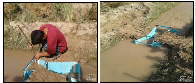
Fig 2: Discharge measurement from the the upstream of watercourse with cut throat flume installed.
