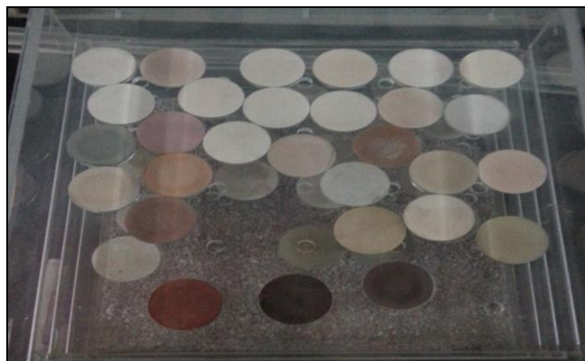
Fig 4: Pressed pellets of samples prior to their analysis by (EDXRF)
