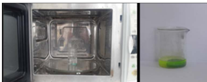
Fig 8: Disinfection of test specimens. a) Microwave irradiation. b) 2% glutaraldehyde disinfection
