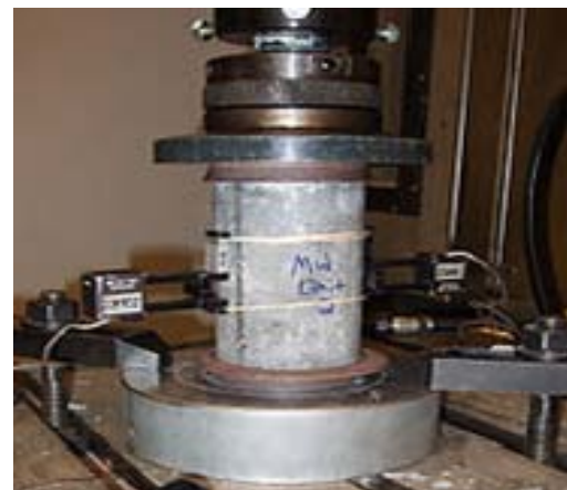
Compression testing of a concrete cylinder
