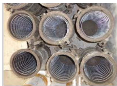
Fig 2: Wire Mesh In The Mould Cylinder
