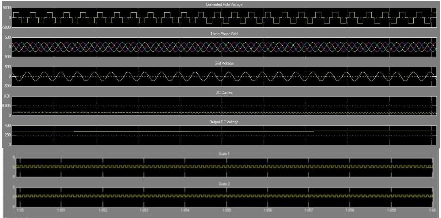
Fig 7: Simulation Steady state waveform under 430/2 KW operation, Converted pole voltage, three phase grid, grid voltage, output DC voltage, Gate pulses respectively.
