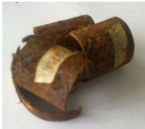
Fig. 2: Corroded pieces of galvanized steel cut and submerged in insitu sea water
