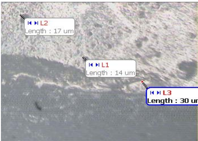
Fig 3: measurement of coating thickness at various points for 5X magnification at low rotational speed
