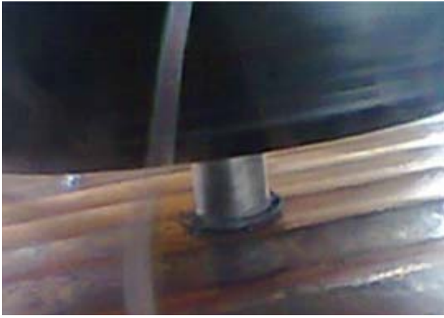
Fig 2: Surface coating using friction surfacing
