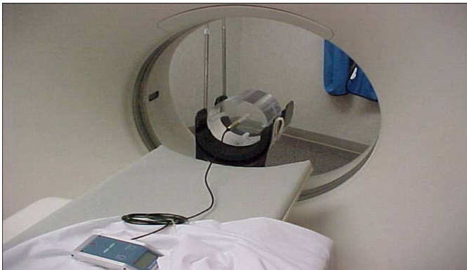
Fig 1: A scanner, phantom with ionization chamber placed in the central insert and an electrometer.
