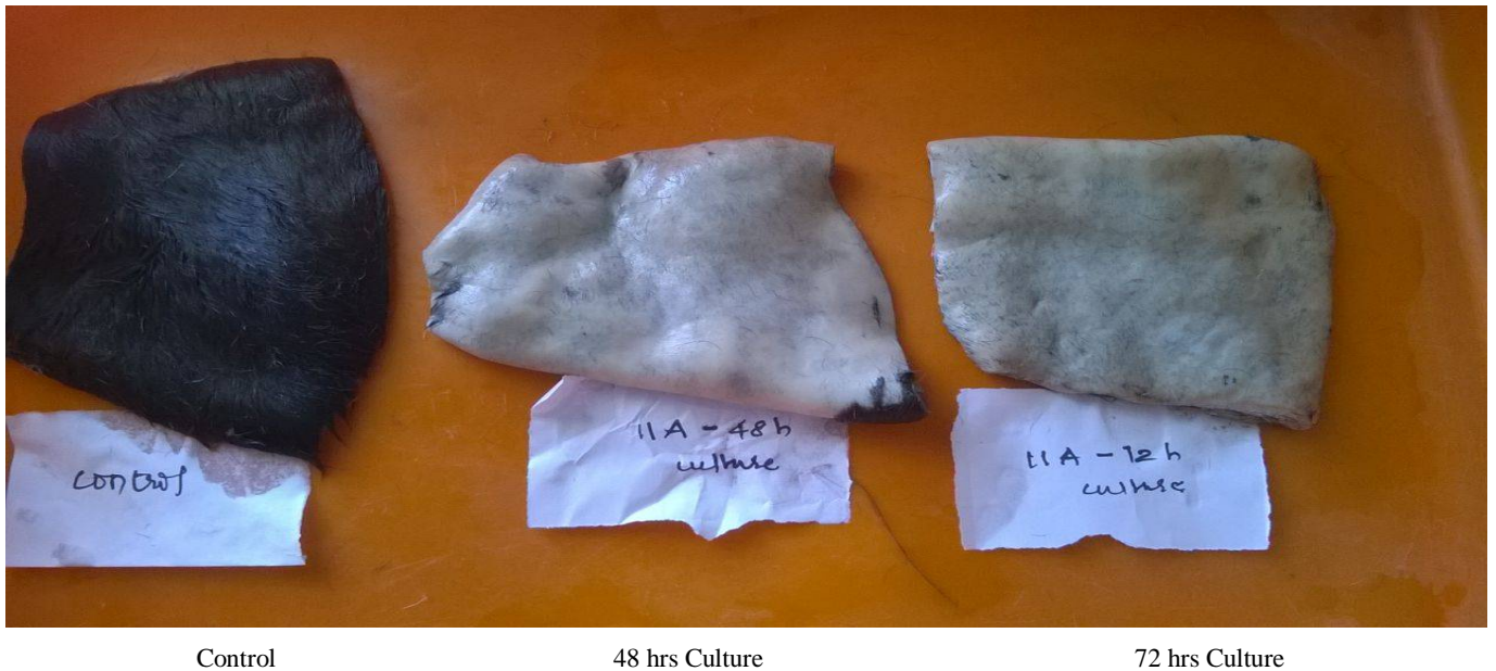
Fig 3.3.3: Direct De-Hairing Activity of the enzyme isolated from Bacillus vallismortis (11A)
