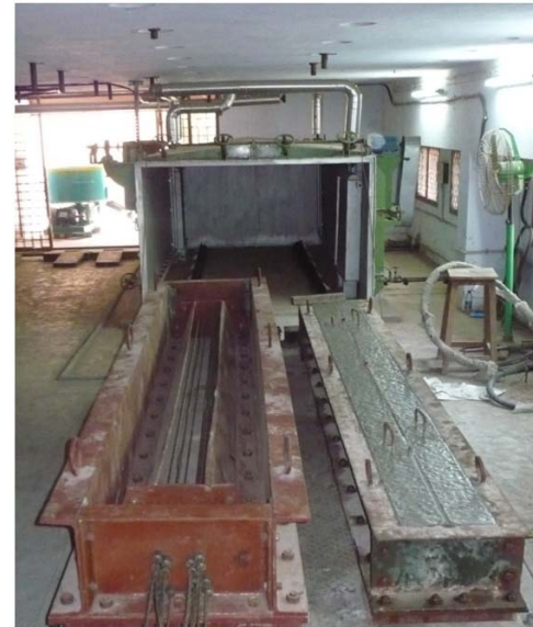
Fig 4.5: Specimens placed in steam curing chamber
