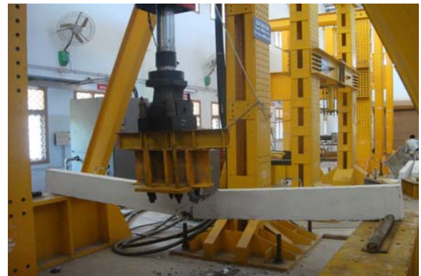
Fig 5.7: Failure pattern of conventional concrete beam
