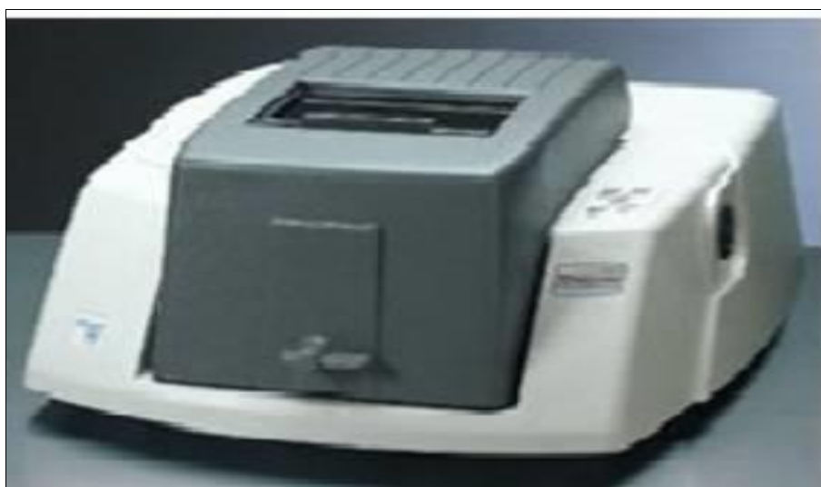
Fig 1: Nicolet Avatar FTIR Spectrometer
