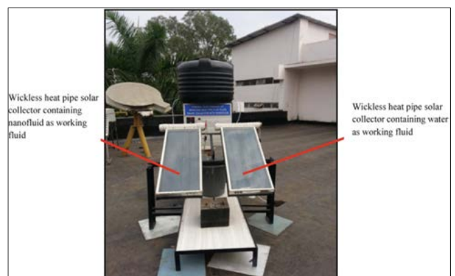
Fig 1: Wickless Heat Pipes structured solar water heater
