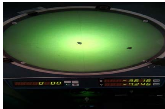
Fig 2: SiC particulate fibres with particle size 343micron.
