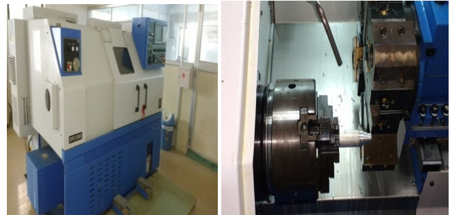
Fig 3: Machining Set Up (Super Jobber CNC Turning)
