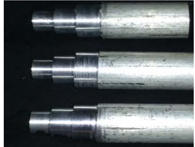
Fig 2: Job material (step turned Al)
