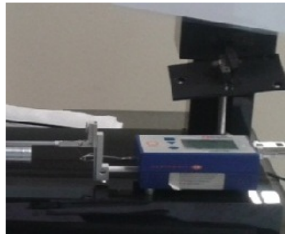
Fig 4: Shows the Talysurf surface roughness testing device for measurement of surface roughness (Ra)
