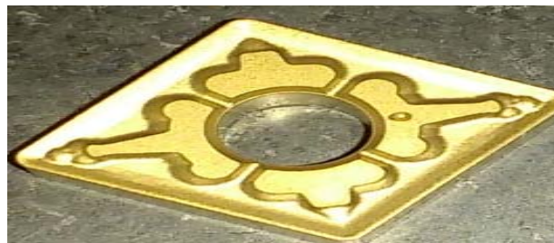
Fig 1: Cutting tool (carbide tipped tool CNMG120408TM-T9125)
