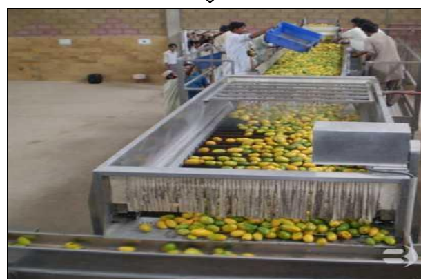
Fig 5: Washing section (removal of dirt or other extraneous matters)
