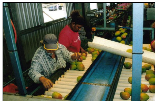
Fig 4: Sorting section (ripe mangoes are sorted out here)
