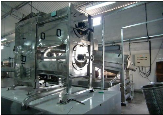
Fig 8: Pulper (making of smooth pulp)
