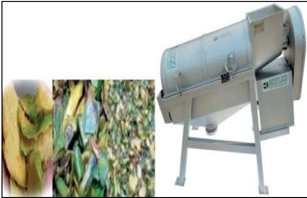
Fig 7: Destoner (peel separation and pulp recovery)
