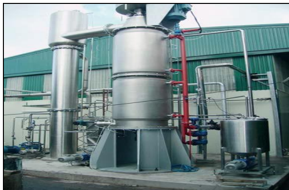
Fig 12: Evaporator (excess air removal & concentration of juice)
