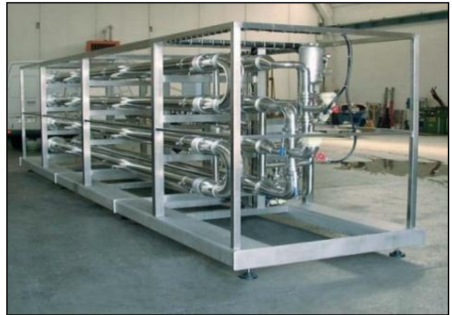
Fig 11: Preheater (enzymatic deactivation)
