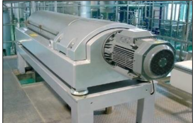
Fig 10: Separator (separation of black specks)
