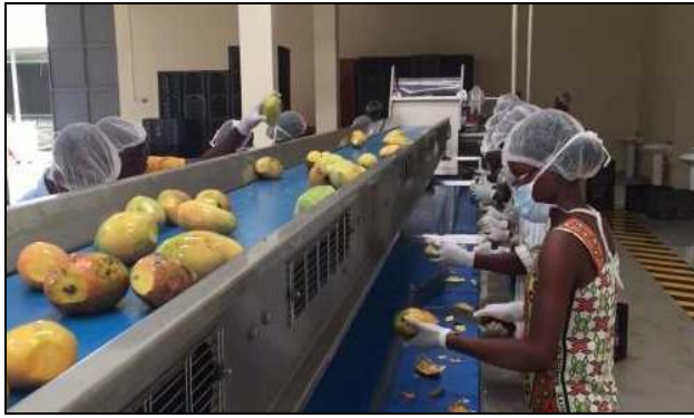
Fig 6: Cutting belt (mango tips are cut here)
