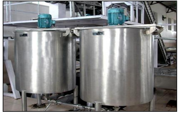
Fig 9: Mixing tank (mixing of additives)
