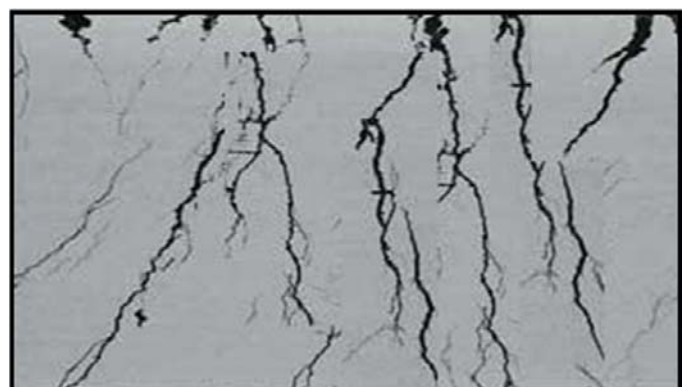
Plate 5a: Micrograph of specimen tensed to 253.6N/m^2 for a period of 360 hours in 1MH_2SO_4 environment. (x500), temp ( 25^\circ C ).
