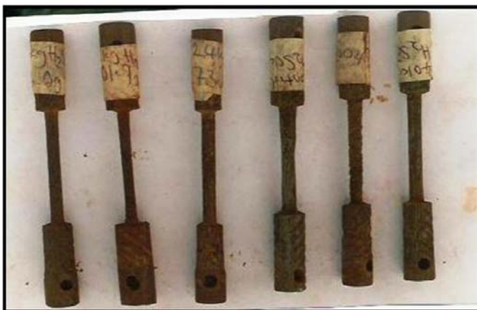
Plate 1: Macrograph of specimens tensed to various levels of stress in 1MH_2SO_4 environment.
