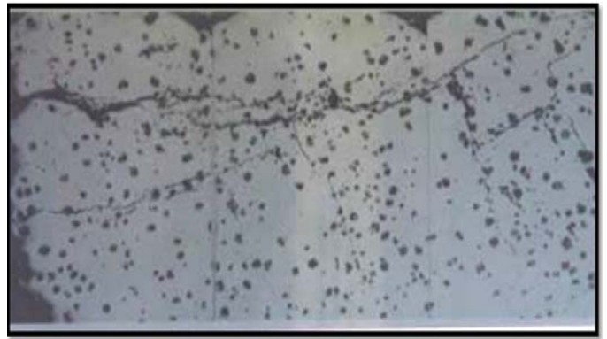
Plate 6a: Micrograph of specimen tensed to 253.6N/m 2 for a period of 360 hours in 1MHCl environment. (x500), temp (25 °C).
