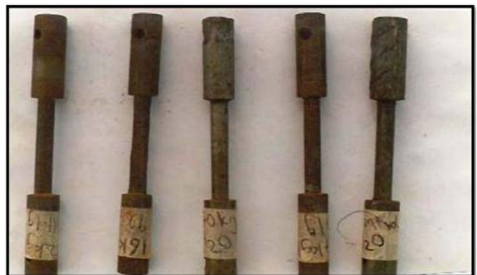
Plate 4: Macrograph of specimens tensed to various levels of stress in H_2O environment.
