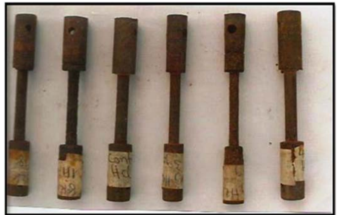
Plate 2: Macrograph of specimens tensed to various levels of stress in 1MHCl environment.
