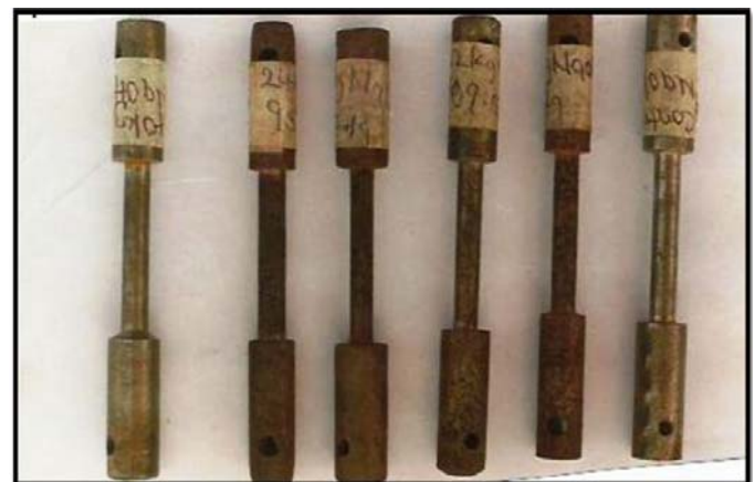
Plate 3: Macrograph of specimens tensed to various levels of stress in 1MNaOH environment.
