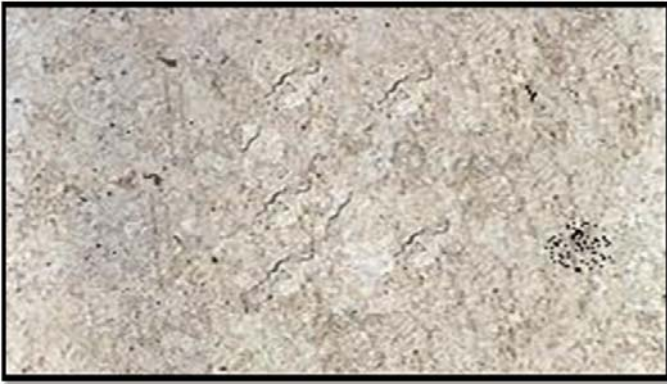
Plate 6e: Micrograph of control specimen immersed in 1M HCl environment for a period of 360 hours. (x500), temp (25 °C).
