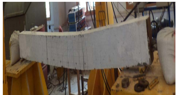
Fig 11: Crack Pattern of GPC Post Tensioned Beam
