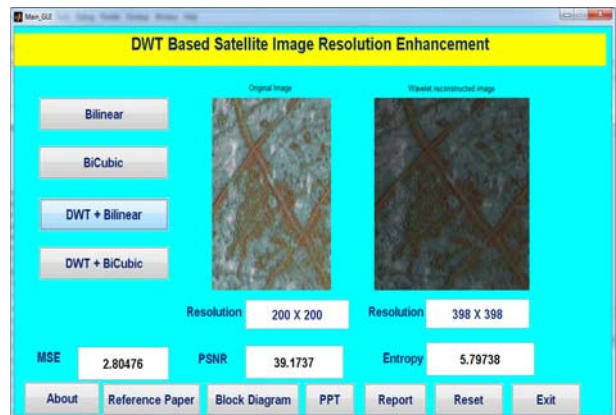
Fig 4.3: DWT- Based Bilinear Interpolation and Result parameter
