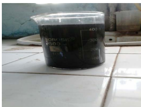
Fig 1.a) solution of reducing agent and AgNO 3 b) after addition of metal solution and reducing agent
