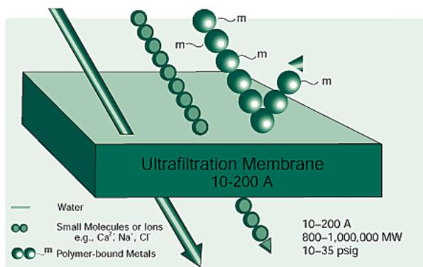
Polymer Filtration is a membrane-based technology for metal-ion recovery. This separations technology uses specially designed, water soluble polymers that selectively bind metal ions to prevent metals from entering waste water streams and to prevent sludge formation.
