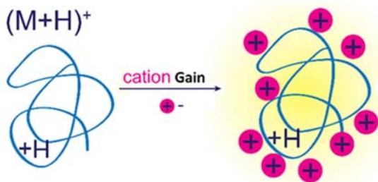
Above diagram shows the activation of the polymer surface by gaining the cation and activation of the specific sites. M shows the polymer matrix and H<sup>+</sup> shows its tendencies to accept or gain cation. This charging process is done in the an non-polar solvent to accumulate a homogeneous activation on the solute i.e. the polymer chain surface.
