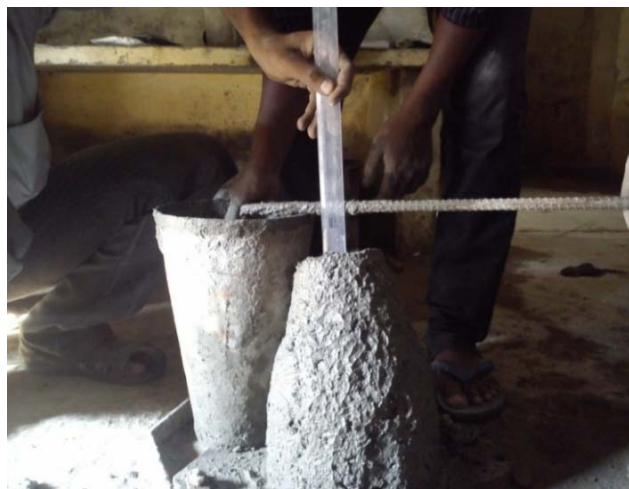
Fig 3.5: Slump test on concrete
