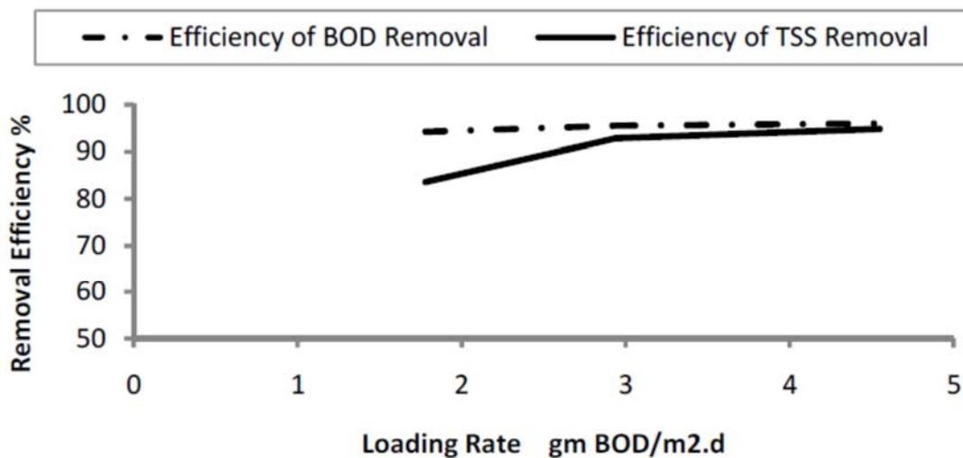
Figure 8 Relation between loading rate and removal efficiency
