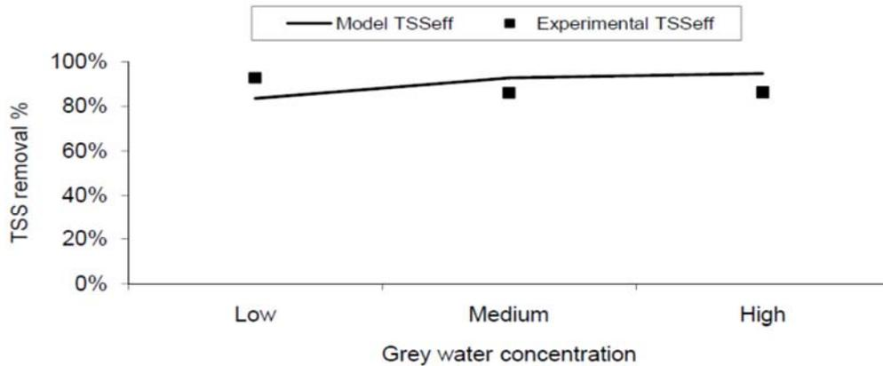
Figure 6 Relation between grey water concentration and TSS removal efficiency.
