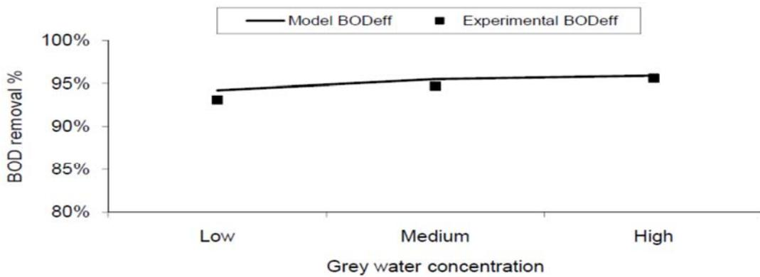
Figure 7 Relation between grey water concentration and BOD removal efficiency
