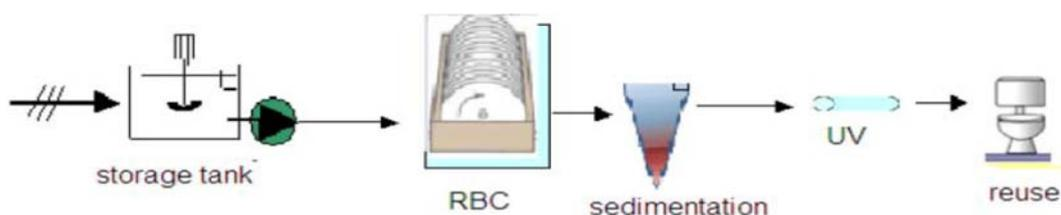
Figure 2 Schematic illustration of the RBC experimental system
