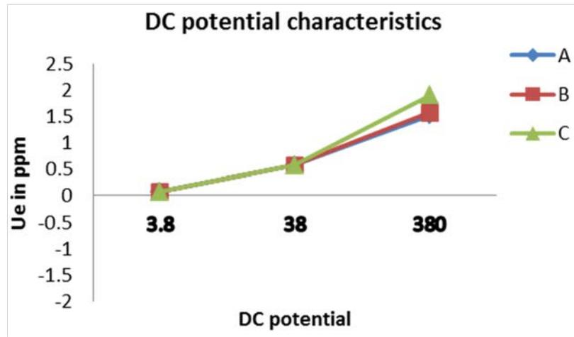
Fig 5: Uncertainty of dc potentials of Multimeter
