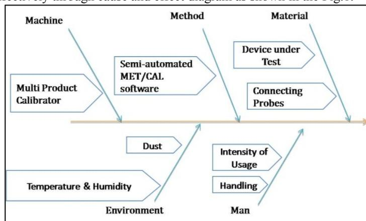
Fig 1: Cause and Effect diagram
