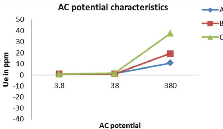
Fig. 4: Uncertainty of ac potentials of Multimeter
