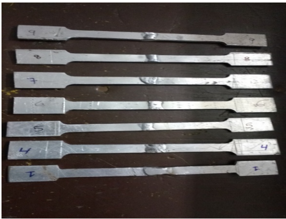
Fig 4: Configuration of Tensile Specimen by GTAW
