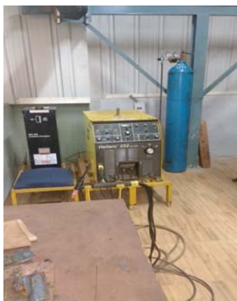
Fig 1: Set-up of GTAW
